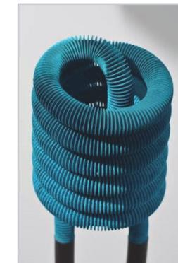
**MOF-coated heat exchanger (Fraunhofer ISE)**
